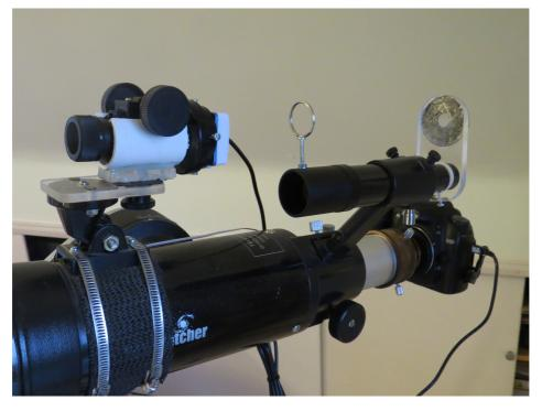
This is the complete kit of parts showing the gunsights on the spotting scope and the webcam spotting scope mounted on a tilt head
